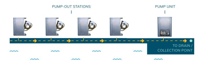
If your harbour need several pump-out stations you only need one main pump unit to manage all the stations. The pump unit will be scaled to the number of stations you need.
